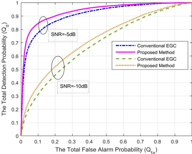
Fig. 4. The ROC for conventional EGC and proposed methods
