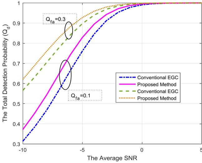
Fig. 3. The total detection probability versus average SNR
