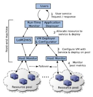
Fig. 2. Architecture DeSVI and components
