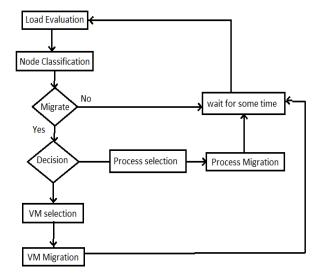
Fig. 2. Flowchart of different phases of algorithm
