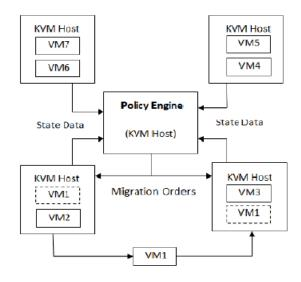
Fig. 3. Architecture containing cluster nodes and central host [4]
