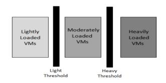
Fig. 1. Each node is assigned one of three regions. Darker region indicates more load on node
