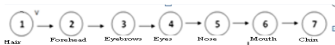
Fig. 4: A one dimensional HMM model with seven states for a face image with seven regions
