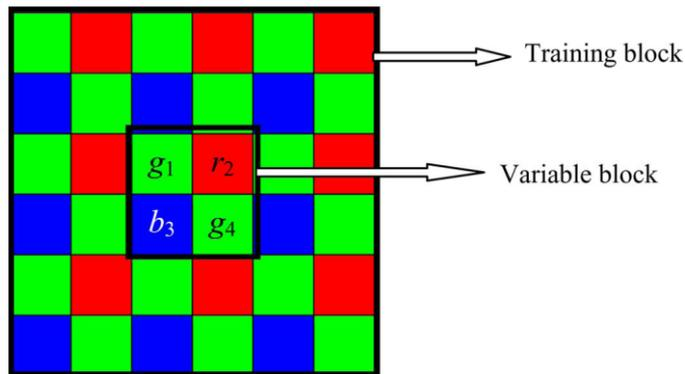
Figure 3. Variable block and training block in the spatially adaptive PCA-based CFA image denoising. Image taken from [1]
