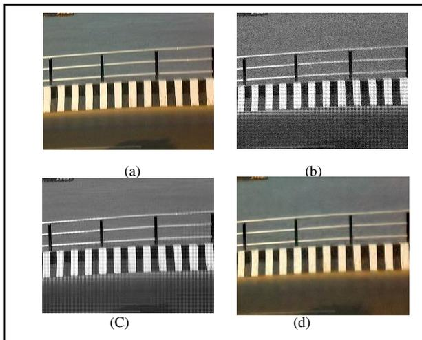
Figure 5. Image 1 (a) Original image (b) Noisy image (c) Denoised Image (d) CDM image
