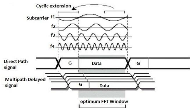
Figure 1: Cyclic Prefix Insertion in the Guard Band
