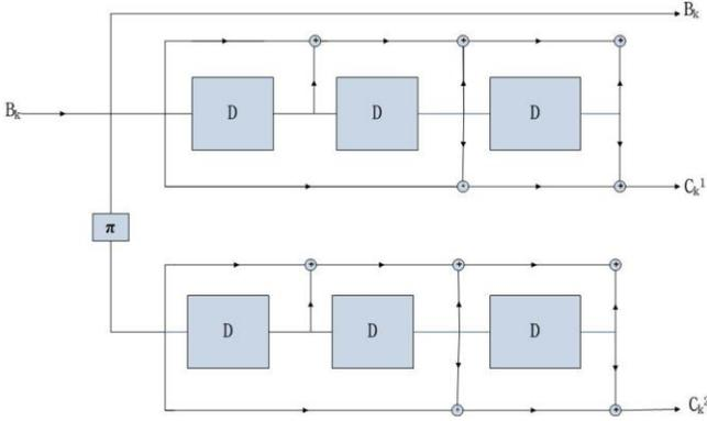
Figure 5: Turbo Encoder with code rate of 1/3
