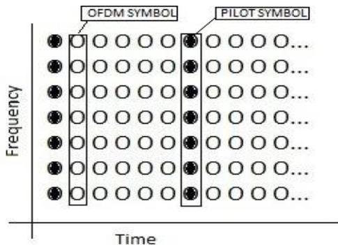
Figure 4: Block-type pilot symbols within OFDM symbols
