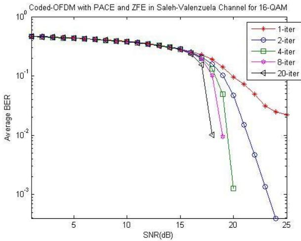
Figure 11: Curves for different iterations of Log-Map Decoder for 16-QAM in SV channel with AWGN
