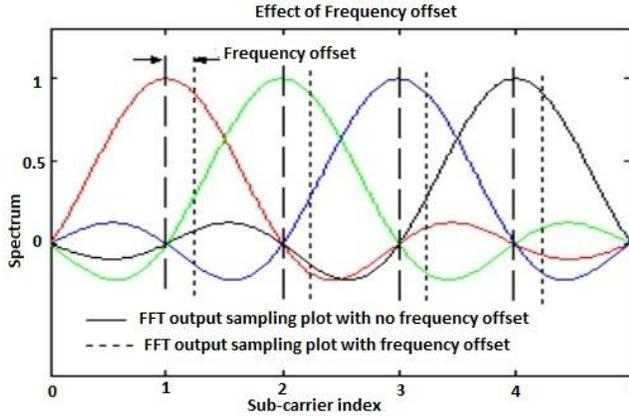
Figure 2: Frequency offset introduced by ICI
