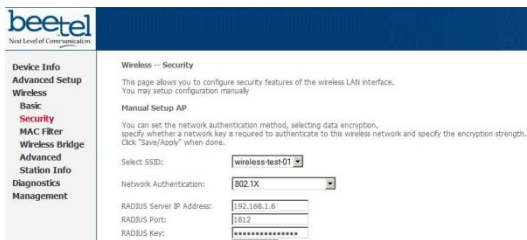
Fig. 5: Beetel 450BXI Router configured in 802.1X Network Authentication with Shared Key (same as Radius server)
