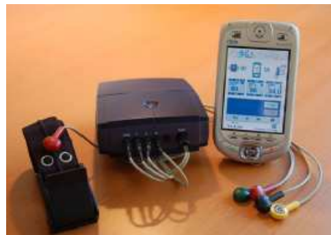
Fig. 2. BAN with electrodes and respiration sensor
