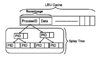
Fig. 4. Block diagram for LRU cache with Splay tree
