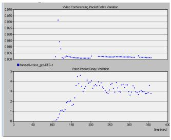
Fig. 2: Packet delay variation under GRP
