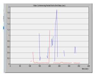
Fig. 5: End to End delay on video traffic for AODV and GRP
