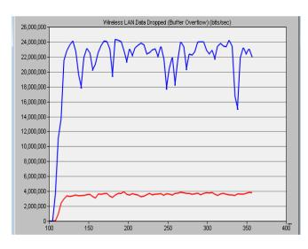
Fig. 3: Data dropped due to buffer overflow
