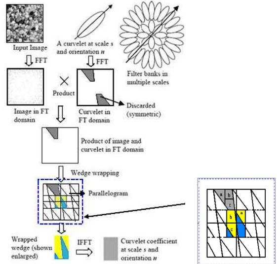
Fig. 3. Image to Curvelet coefficients
