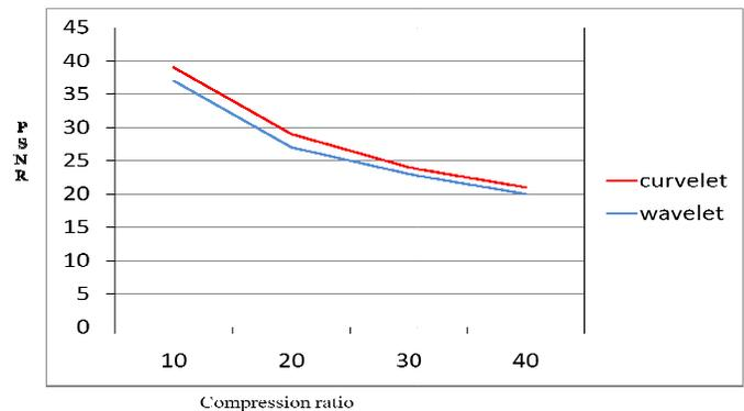
Fig. 8. Comparison of wavelet and proposed algorithm compression ratio with PSNR
