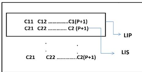
Fig. 5. List Formations in Modified SPIHT Algorithm
