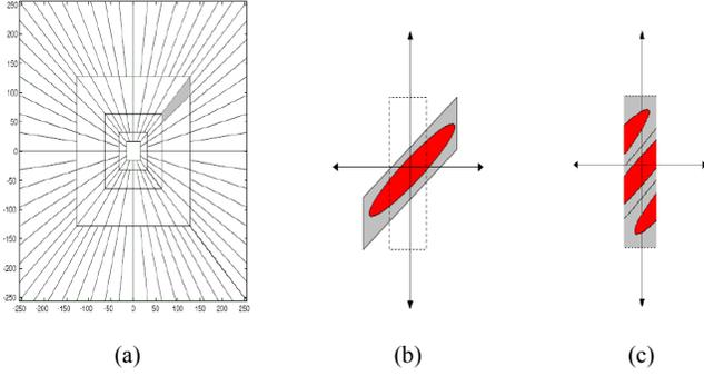
Fig. 2. (a) Digital Corona of the Frequency Domain, (b) Support of Wedge before Wrapping; and (c) Support of Wedge after Wrapping
