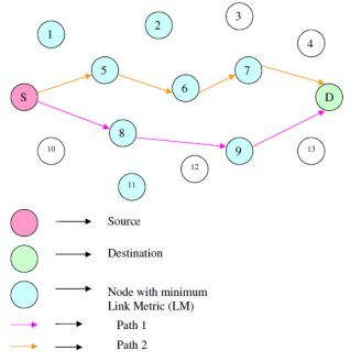
Fig. 1. Multipath Establishment using Multipath Dijkstra Algorithm
