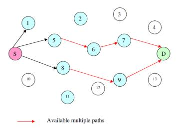
Fig. 3. Reactive Multi-path Routing
