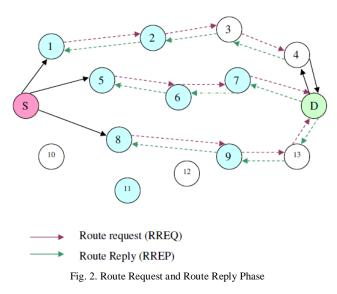
From Fig. 2, the intermediate node 5, 1, 8 starts broadcasting RREQ packets. Upon receiving the RREQ packet, the neighbor nodes reply with the RREP packet to the requested node. The node 5, 1 and 8 verifies the RREP and computes its link metrics and if the link metrics matches with the value already stored in its TIT, it start sending data following that route and discard other duplicate RREP packets.
