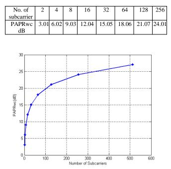
Figure 1. PAPR<sub>WC</sub> versus number of subcarriers
