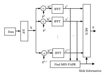
Figure 2. The structure of transmitter with SLM scheme
