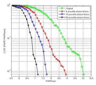
Figure 11. CCDF comparison of PTS with different number of phase factors
