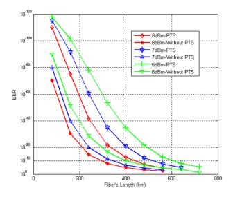
Figure 13. BER of long haul optics fiber link with PTS algorithm
