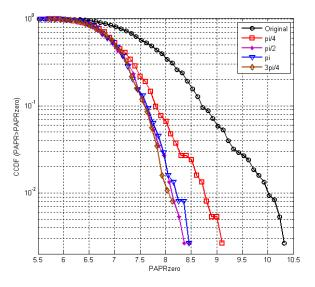
Figure 10. Rotation phase dependence of SLM incase of 4 sub-blocks
