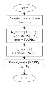
Figure 5: Flowchart of Optimization sub-system
