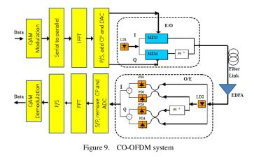
At the receiver, after converting the signal from optical to electrical domain by using photo-detectors, the electrical signal is processed to give back the data via de-OFDM modulation and 4-QAM de-modulation.
