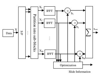
Figure 4. The structure of transmitter site with PTS
