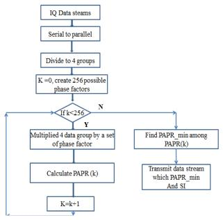
Figure 3. SLM algorithm flowchart
