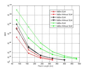
Figure 12. Performance of long haul optics fiber link with SLM
