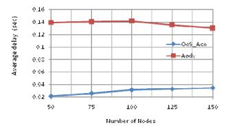
Fig. 1. Average End to End delay, density of nodes
