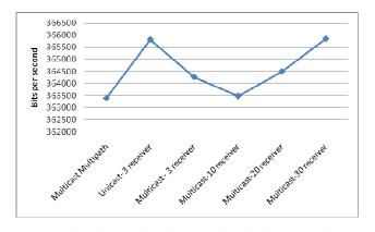
Fig. 5: The mean throughput at receiver F in bits per second
