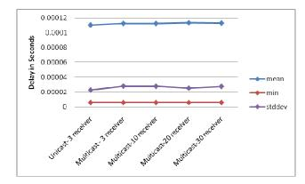
Fig. 3: The queuing delay in seconds at the backbone router as it receives traffic from sender.
