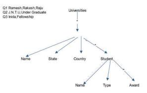
Fig. 1: Schema of an XML Document
