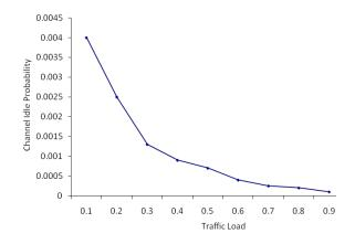
Fig. 5: Channel Idle Probability against Traffic Load
