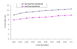
Fig. 8: Average delay against system throughput
