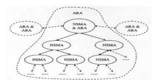
Fig. 2. Sub-HST: Construction of ARA (Autonomy Represented by Agent) (NSMA: Node State Monitoring Agent)
