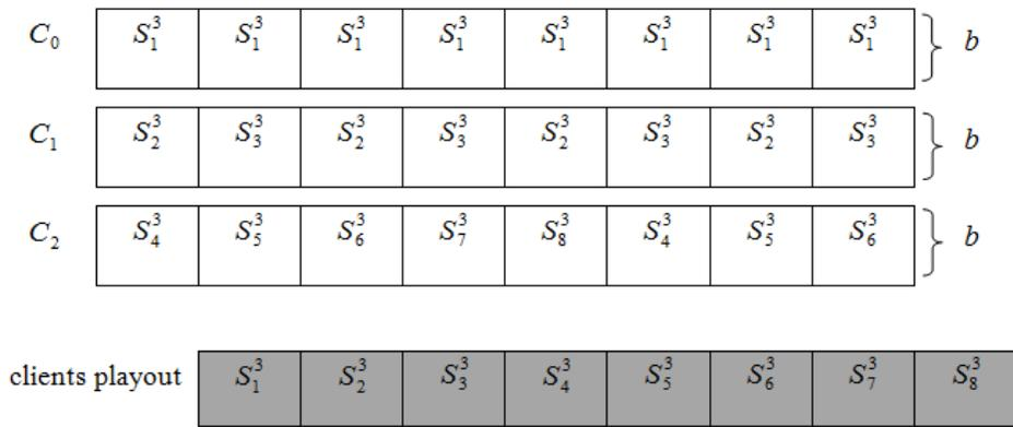
Fig. 2. The channel allocation for Buffer Efficient Fast Broadcasting (BEFB) Scheme with  $k=3$
