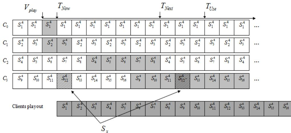
Fig. 3. An illustration of segment downloading for BEFB scheme
