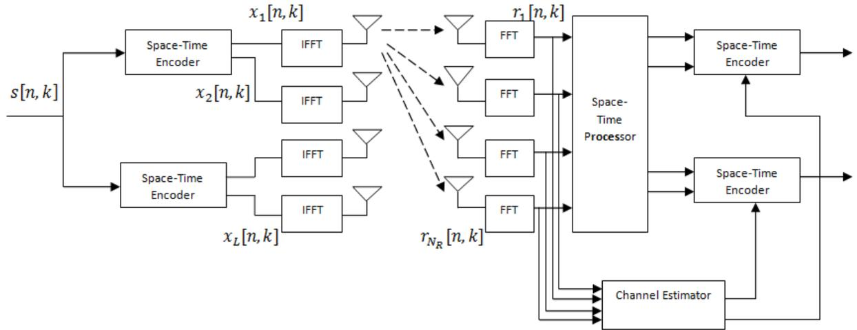
Fig.1: MIMO-OFDM System Model [7]
