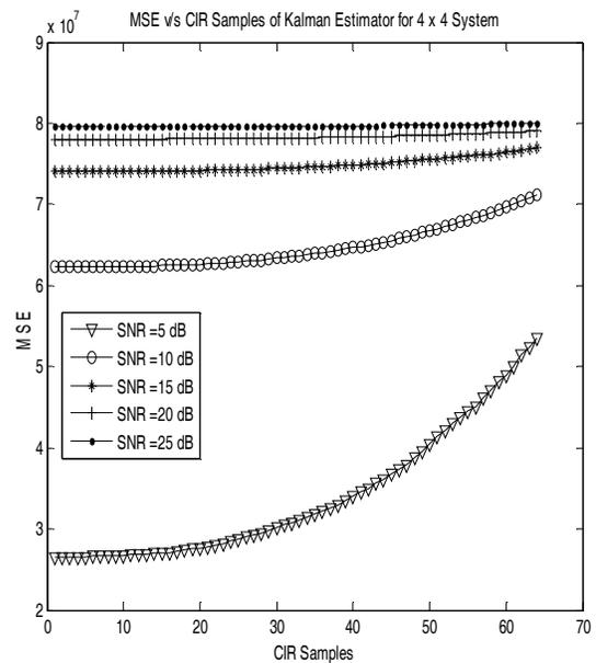
Fig. 2: MSE vs CIR Samples of Kalman Estimator for  $4 \times 4$  System
