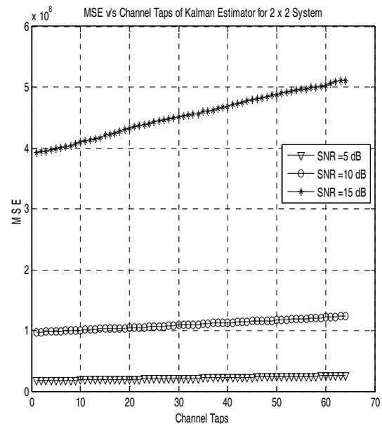
Fig. 6: MSE vs Channel Taps of Kalman Estimator for  $2 \times 2$  System
