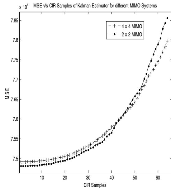
Fig. 3: MSE vs CIR Samples of Kalman Estimator for different MIMO Systems
