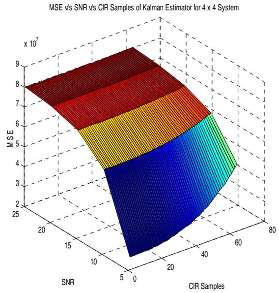
Fig. 5: MSE vs SNR vs CIR Samples of Kalman Estimator for  $4 \times 4$  System
