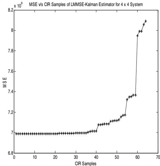
Fig. 4: MSE vs CIR Samples of LMMSE-Kalman Estimator for  $4 \times 4$  System
