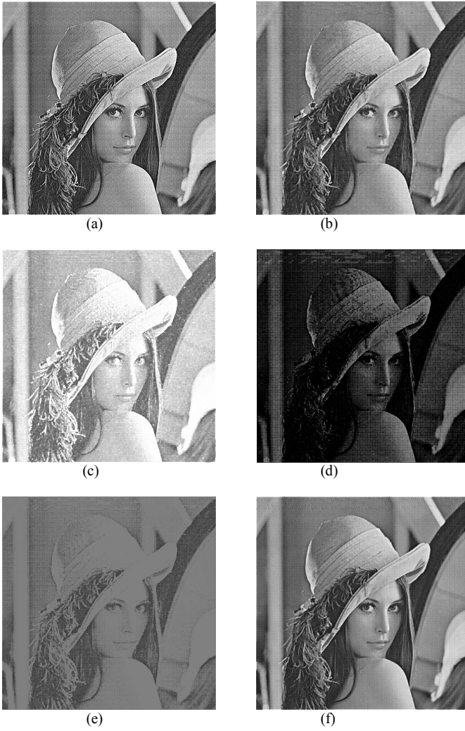
Fig. 4. Filters Attack on Comparison Based Watermarking Techniques using WGN (a) Original watermarked image (b) Watermarked image after median filter (c) Watermarked image after max filter (d) Watermarked image after min filter (e) Watermarked image after midpoint filter (f) Watermarked image after alpha-trimmed mean filter
