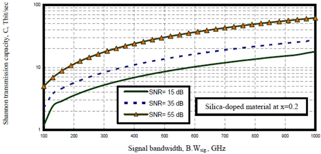
Fig. 20. Variations of Shannon capacity against transmission signal bandwidth at the assumed set of parameters.
