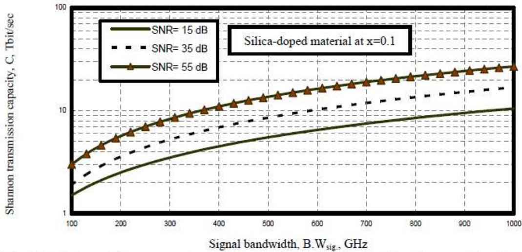
Fig. 19. Variations of Shannon capacity against transmission signal bandwidth at the assumed set of parameters.
