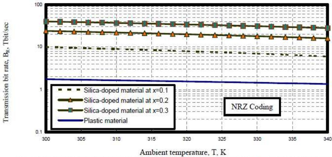
Fig. 11. Variations of transmission bit rate against ambient temperature at the assumed set of parameters.
