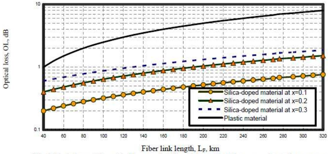
Fig. 2. Variations of the optical loss against fiber link length at the assumed set of parameters.
