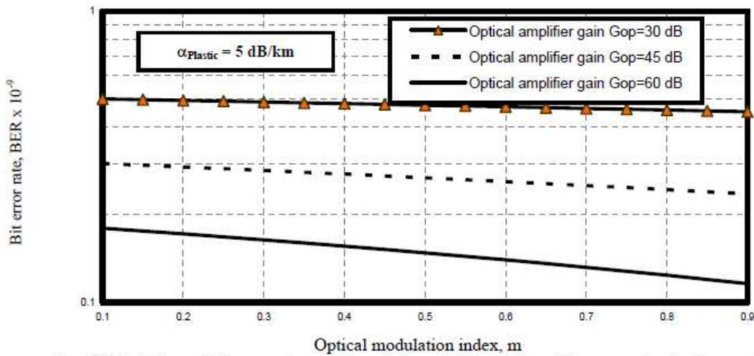
Fig. 10. Variations of bit error rate against optical modulation index at the assumed set of parameters.
