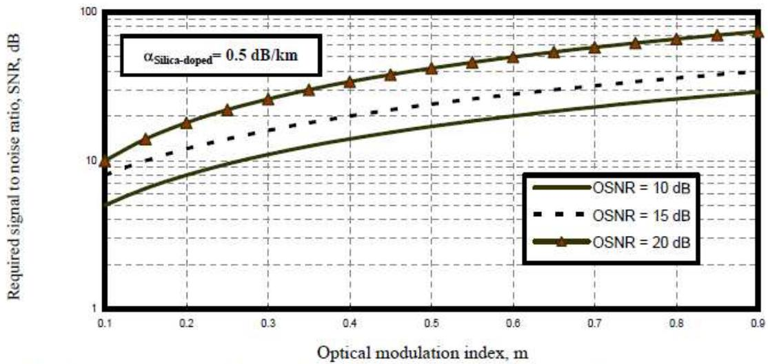
Fig. 3. Variations of signal to noise ratio against optical modulation index at the assumed set of parameters.
