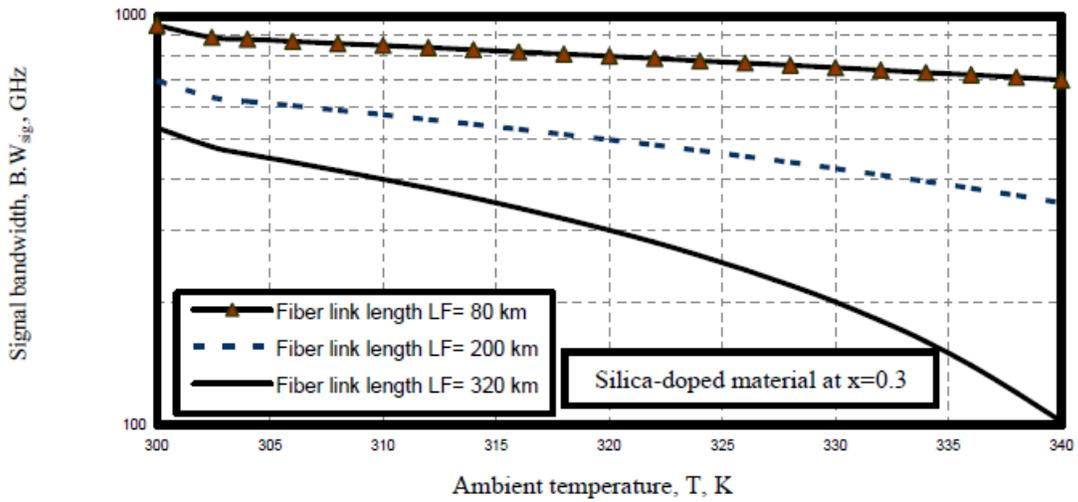
Fig. 15. Variations of transmission bit rate against ambient temperature at the assumed set of parameters.
