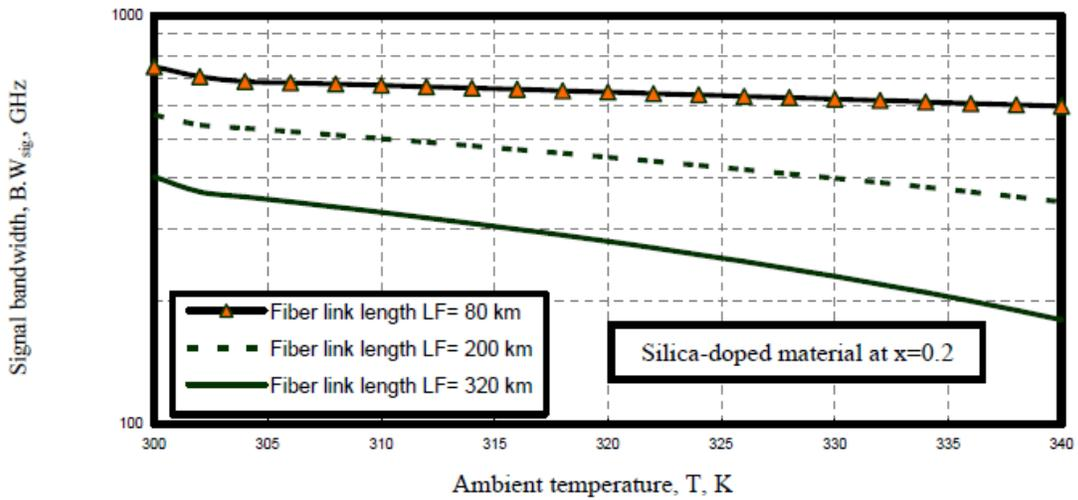
Fig. 14. Variations of transmission bit rate against ambient temperature at the assumed set of parameters.
