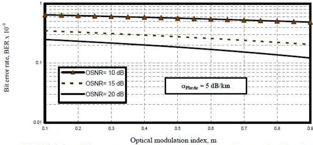
Fig. 8. Variations of bit error rate against optical modulation index at the assumed set of parameters.
