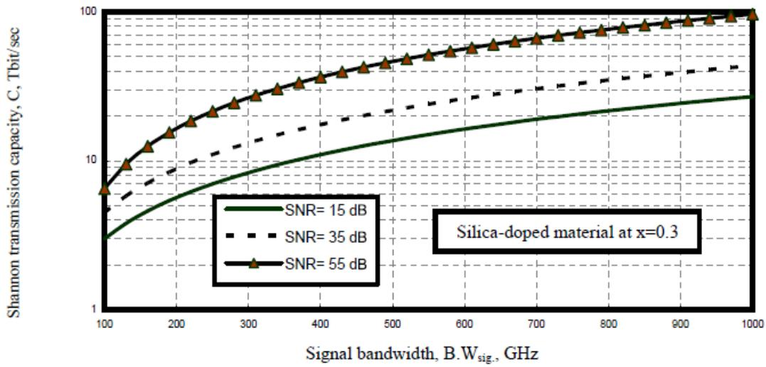
Fig. 21. Variations of Shannon capacity against transmission signal bandwidth at the assumed set of parameters.
