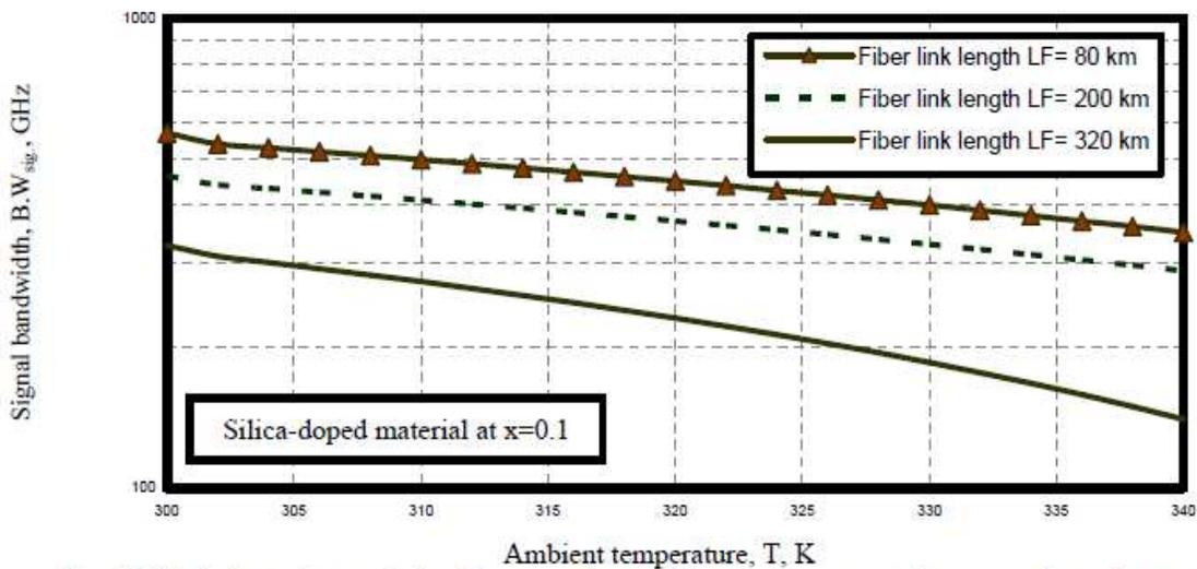
Fig. 13. Variations of transmission bit rate against ambient temperature at the assumed set of parameters.
