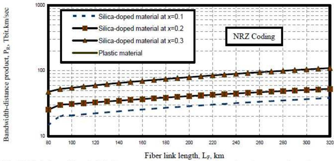
Fig. 17. Variations of bandwidth-distance product against fiber link length at the assumed set of parameters.
