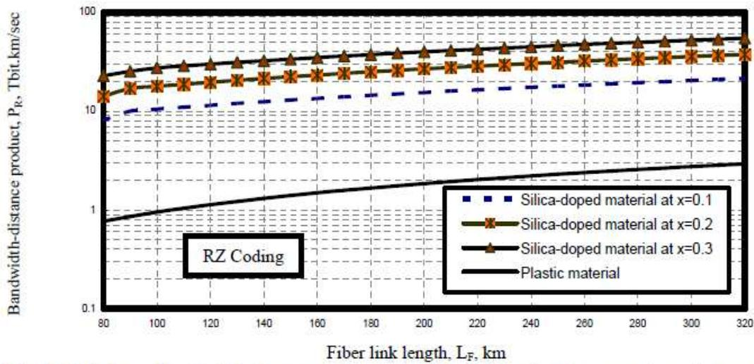
Fig. 18. Variations of bandwidth-distance product against fiber link length at the assumed set of parameters.
