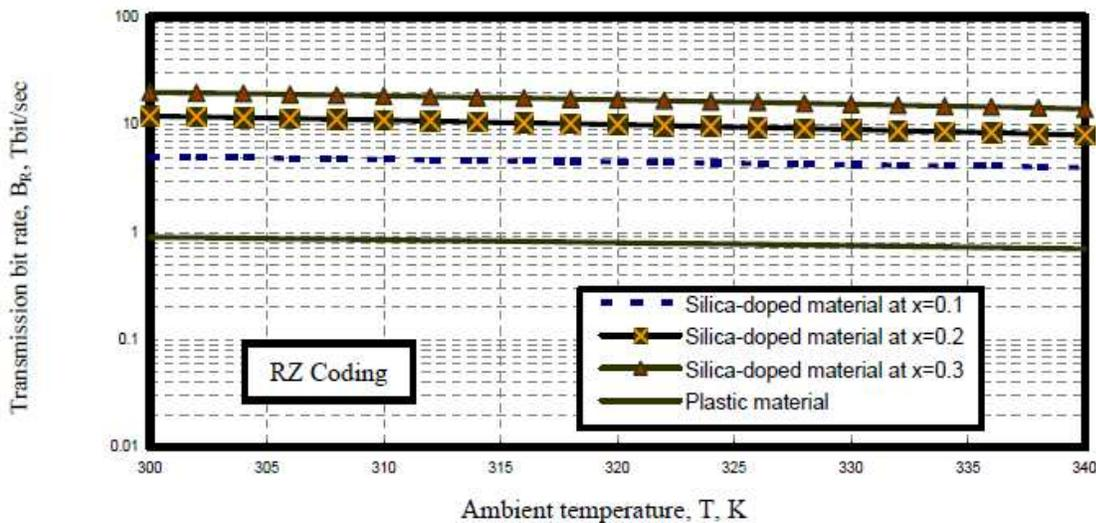
Fig. 12. Variations of transmission bit rate against ambient temperature at the assumed set of parameters.
