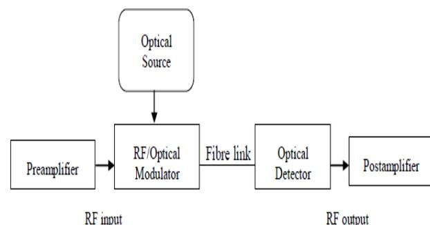
Fig. 1. Intensity modulation direct detection optical link
