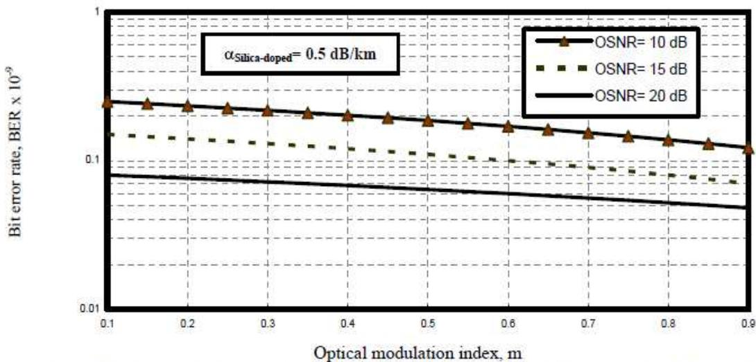
Fig. 7. Variations of bit error rate against optical modulation index at the assumed set of parameters.
