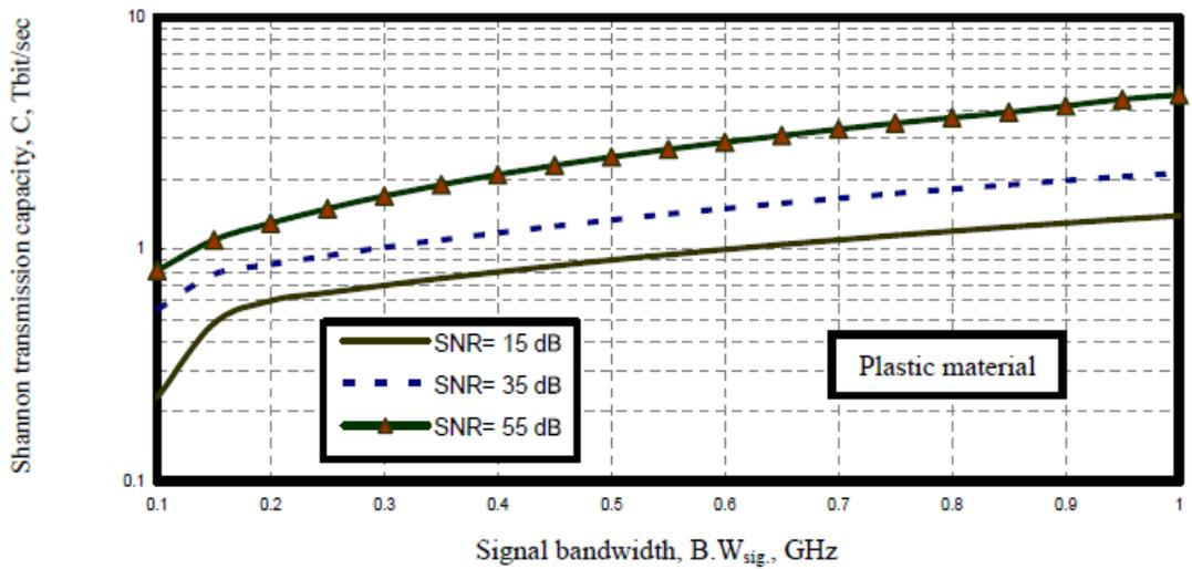
Fig. 22. Variations of Shannon capacity against transmission signal bandwidth at the assumed set of parameters.
