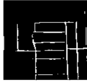
Fig. 9: Extract Road edges from the thinning algorithm
