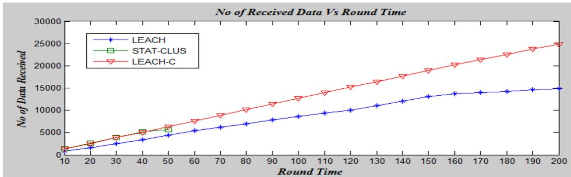
Fig. 7: 50 nodes Scenario for number of Received data at base station vs. Round time
