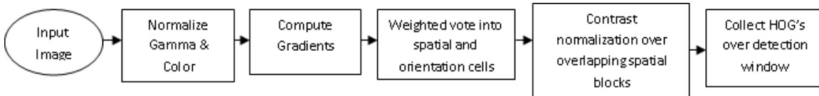
Fig. 3: Block diagram of Histogram of Oriented Gradients
