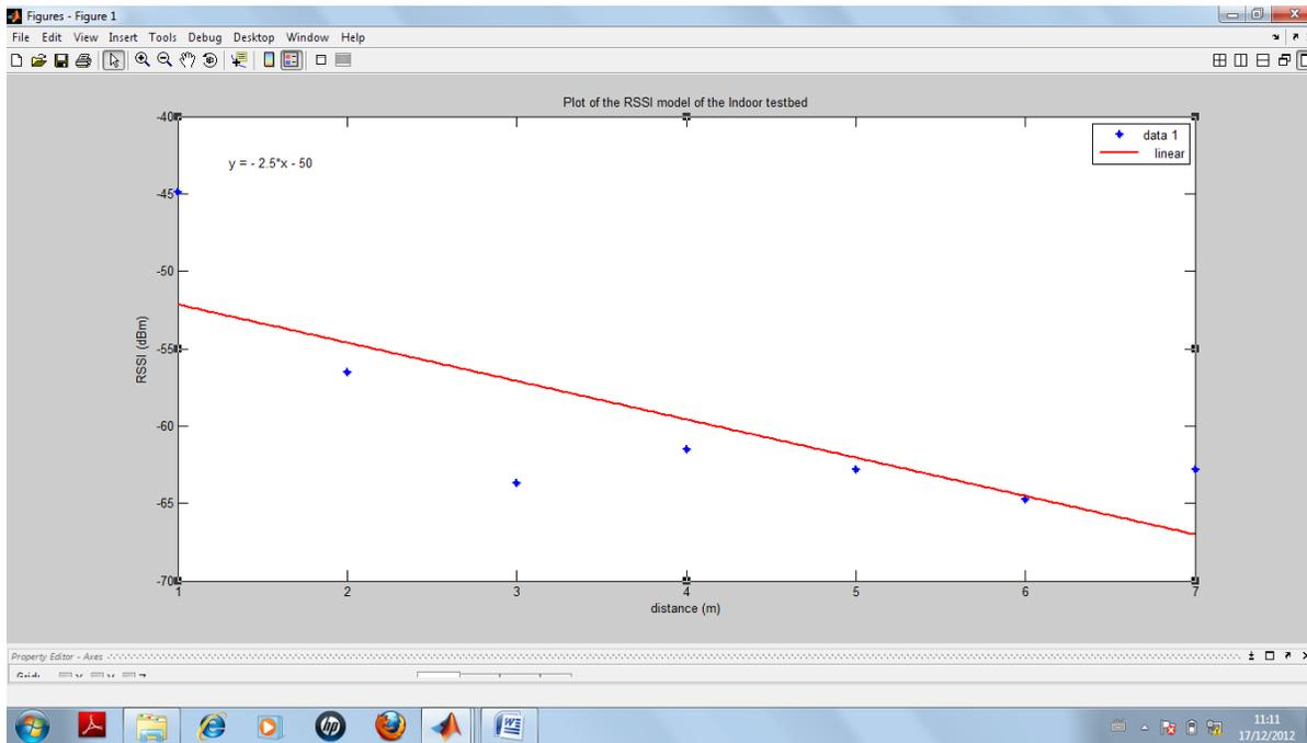
Fig. 5: Plot of the model of the RSSI of the testbed
