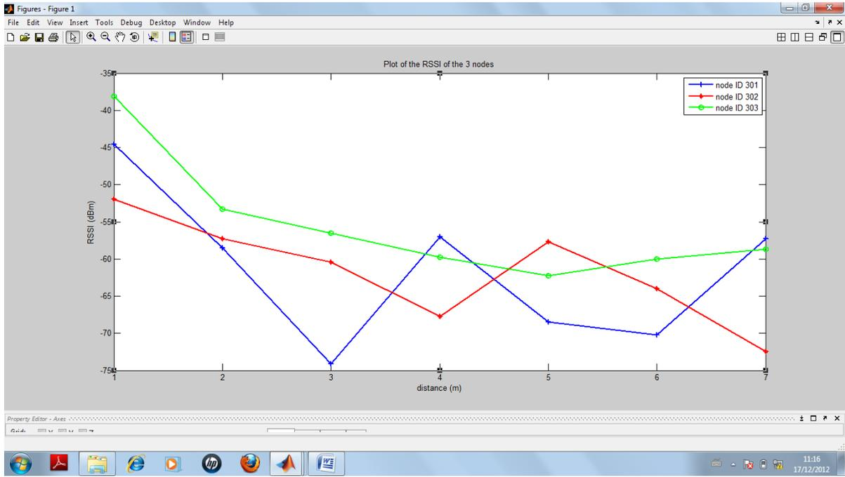
Fig. 3: A graph of RSSI (dBm) against distance of the 3 nodes of the testbed
