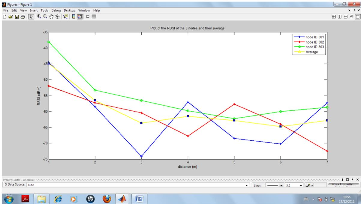
Fig. 4: A graph of RSSI (dBm) against distance of the 3 nodes and their average of the testbed
