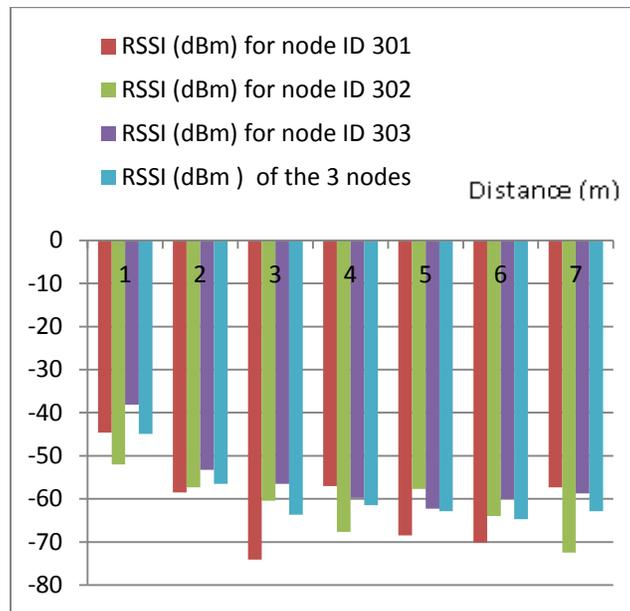
Fig. 2: Bar Chart of the mean RSSI of the three sensor nodes and average
