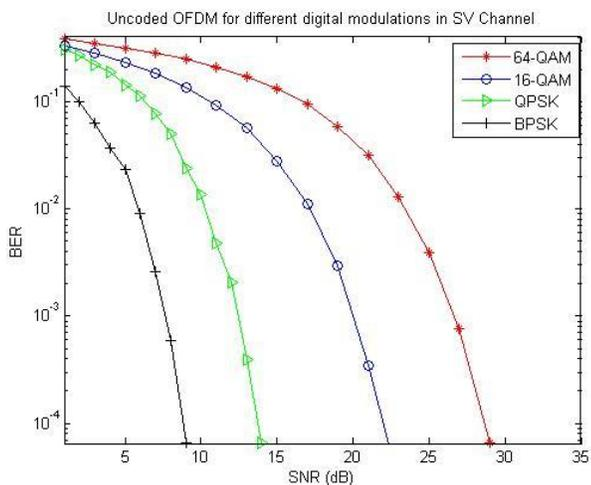
Figure 8: Curves for Un-Coded OFDM in SV channel with AWGN
