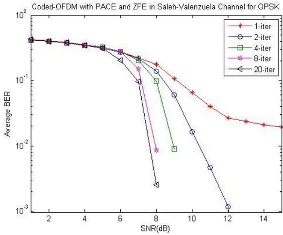
Figure 10: Curves for different iterations of Log-Map Decoder for QPSK in SV channel with AWGN
