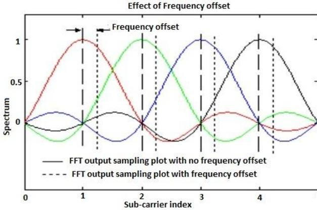
Figure 2: Frequency offset introduced by ICI
