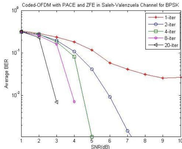
Figure 9: Curves for different iterations of Log-Map decoder for BPSK in SV channel with AWGN
