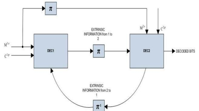
Figure 7: Log-Map Decoder comprised of two elementary Decoders
