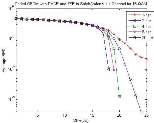
Figure 11: Curves for different iterations of Log-Map Decoder for 16-QAM in SV channel with AWGN
