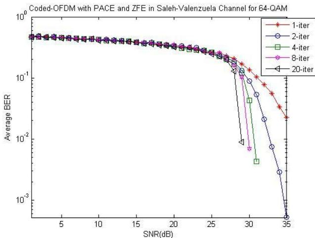
Figure 12: Curves for different iterations of Log-Map Decoder for 64-QAM in SV channel with AWGN
