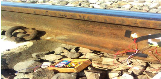
Fig. 5: Actual placement of rolling noise measurement circuit
