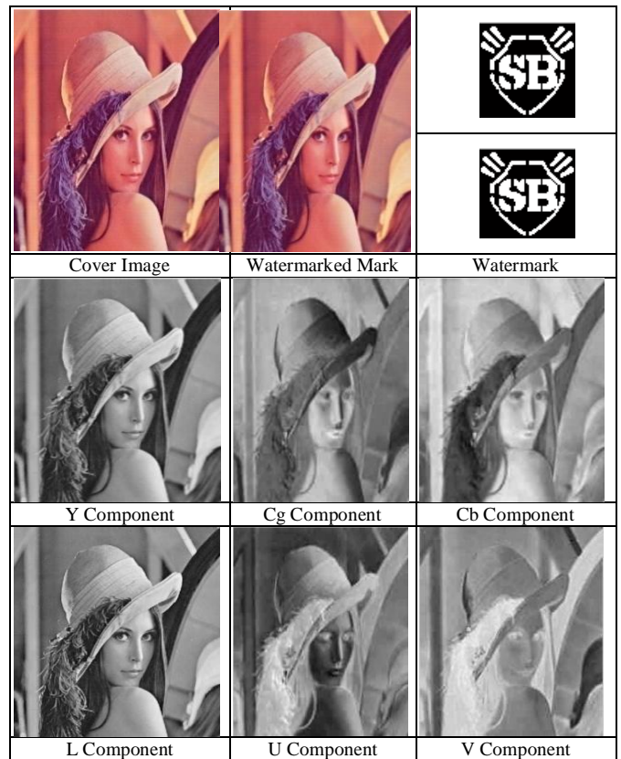
Fig. 7: Various components of 512x512 size Leena Image in YCgCb and YUV Color Space
