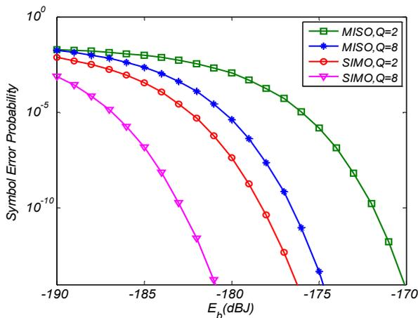
Figure 3. SER vs. bit energy in MISO and SIMO systems with M=N=5 at weak turbulence
