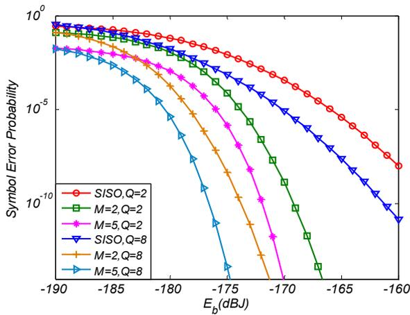
Figure 1. SER vs. bit energy in MISO system at weak turbulence
