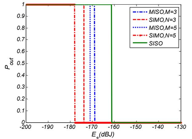
Figure 8.  $P_{out}$  vs. symbol energy in strong turbulence
