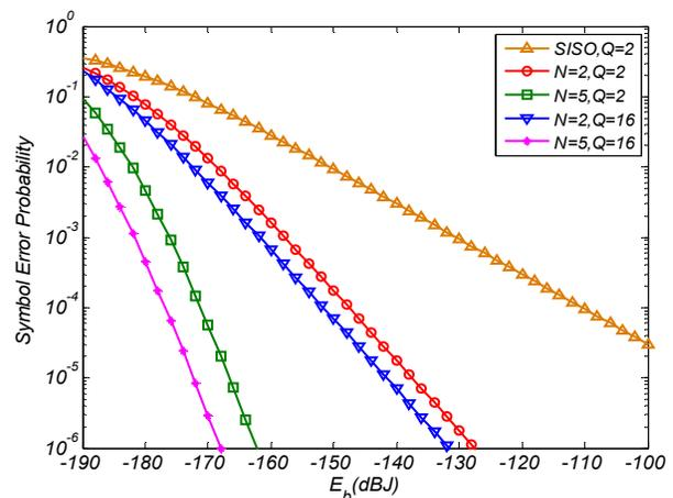
Figure 5. SER vs. bit energy in SIMO system at strong turbulence
