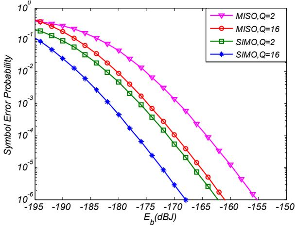
Figure 6. SER vs. bit energy in MISO and SIMO systems with  $M=N=5$  at strong turbulence
