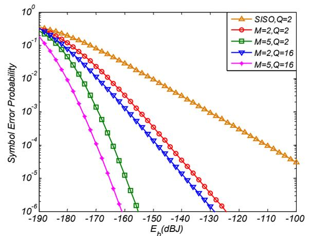
Figure 4. SER vs. bit energy in MISO system at strong turbulence
