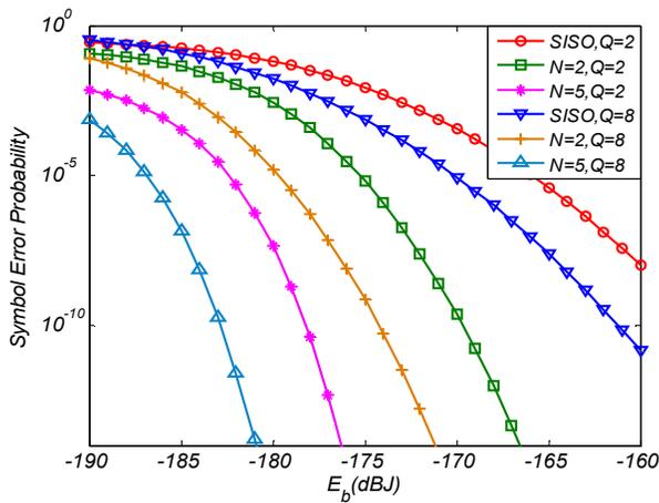
Figure 2. SER vs. bit energy in SIMO system at weak turbulence
