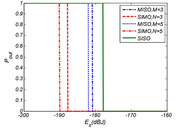
Figure 7.  $P_{out}$  vs. symbol energy in weak turbulence
