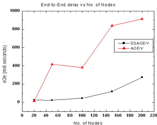
Fig. 3 end-to-end delay vs. Number of nodes
