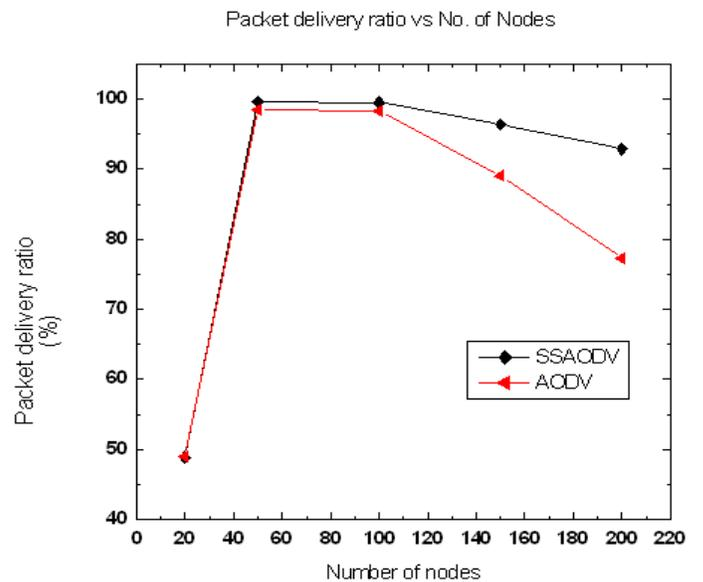
Fig. 5. Packet delivery Ratio vs. Number of nodes
