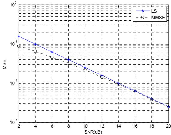
Fig. 7. Channel estimation in 2\*2 MIMO-OFDM systems L=4 with LS and MMSE methods
