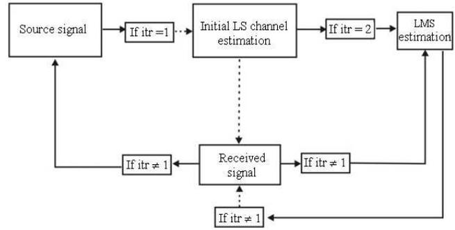
Fig. 4. Implementing LMS algorithm in receiver
