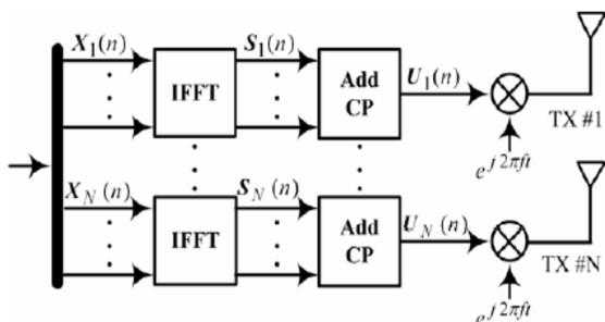
Fig. 2. Diagram block of MIMO-OFDM system's transmitter
