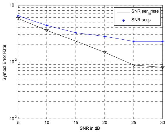
Fig. 6. Plot of SNR V/S SER for an OFDM system with MMSE/LS estimator based receivers
