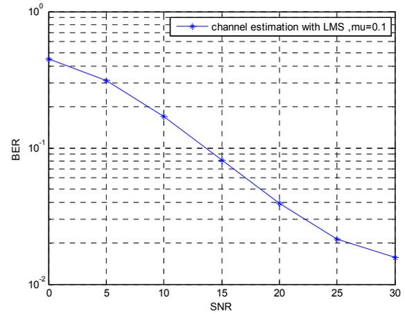
Fig. 14. Channel estimation in 2\*2 MIMO-OFDM systems L=4 with synchronization and LMS algorithm  $\mu=0.1$
