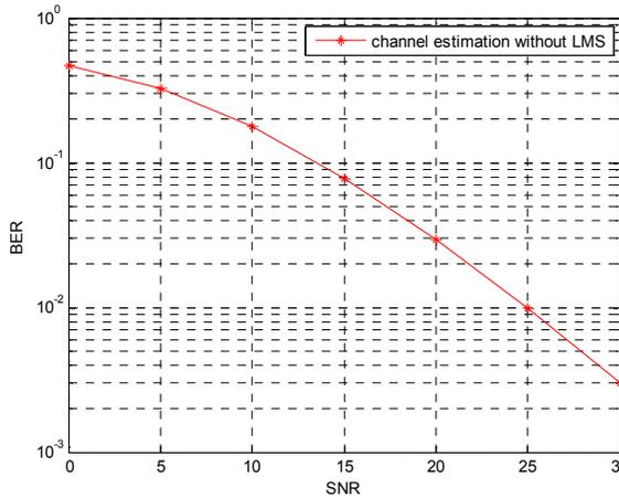
Fig. 12. Channel estimation in 2\*2 MIMO-OFDM systems L=4 with synchronization
