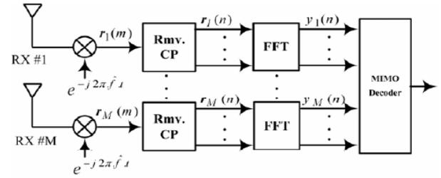
Fig. 3. Diagram block of MIMO-OFDM system's receiver
