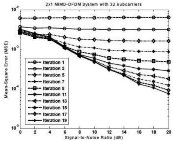
Fig. 9. Mean square error according to SNR for MIMO-OFDM system with 32 sub carriers, which uses 2 transmitter antennas and one receiver antenna with EM algorithm
