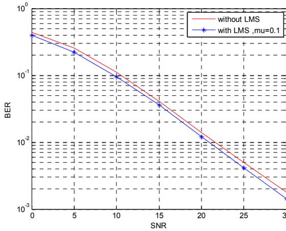
Fig. 11. Channel estimation in SISO-OFDM systems L=5 with synchronization and LMS algorithm  $\mu=0.1$
