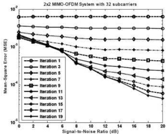
Fig. 10. Mean square error according to SNR for MIMO-OFDM system with 32 sub carriers, which uses 2 transmitter antennas and 2 receiver antennas with EM algorithm
