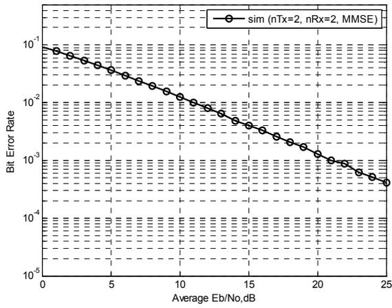
Fig. 5. BER for BPSK modulation with 2x2 MIMO and MMSE equalizer (Rayleigh channel)
