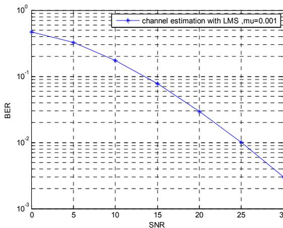
Fig. 13. Channel estimation in 2\*2 MIMO-OFDM systems L=4 with synchronization and LMS algorithm  $\mu=0.001$
