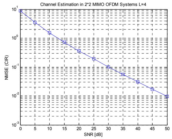
Fig. 8. Channel estimation in 2\*2 MIMO-OFDM systems L=4 without synchronization
