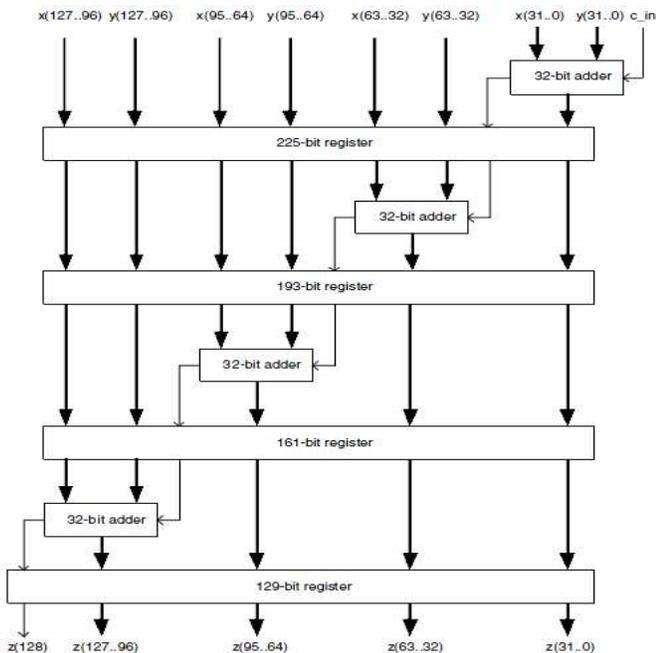
Fig. 4. Pipelined Adder
