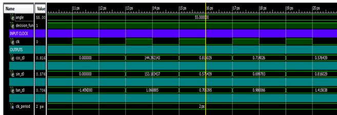
Fig. 6. Simulation result for 32-bit proposed CORDIC
