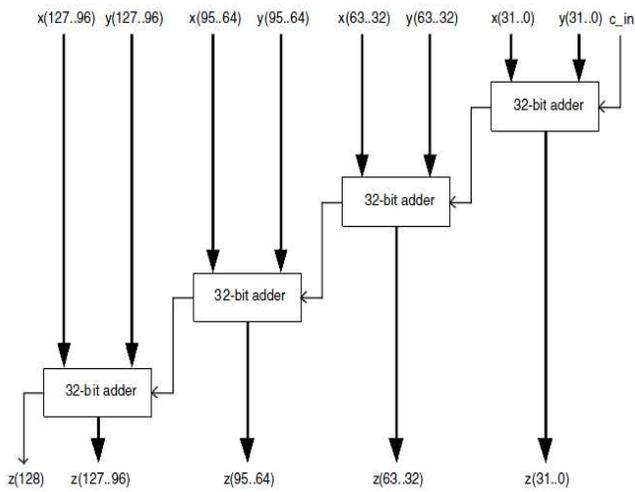
Fig. 3. Parallel Adder
