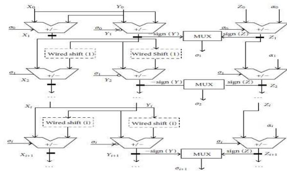
Fig. 2. Unfolded CORDIC design
