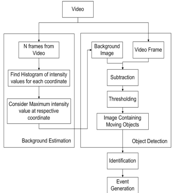
Fig. 2. Block diagram of the proposed algorithm for generating the background image
