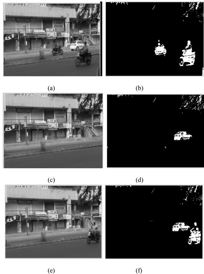
Fig. 10. Result of background subtraction: (a) video frame containing stationary and moving object both, (b) its thresholded image, (c) frame which does not have stationary object, (d) its thresholded image, (e) frame containing only the moving object, (f) its thresholded image
