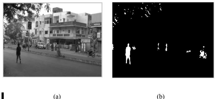
Fig. 5. Result of background subtraction (a) video frame in which car has moved out, (b) thresholded image
