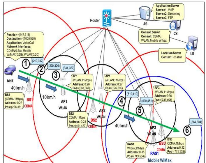
Fig. 3. Simulation environment for handover decisions in CDMA, WLAN, and Mobile WiMax access networks
