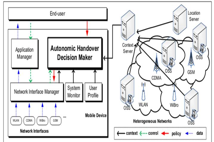
Fig. 2. Terminal management system in heterogeneous wireless network
