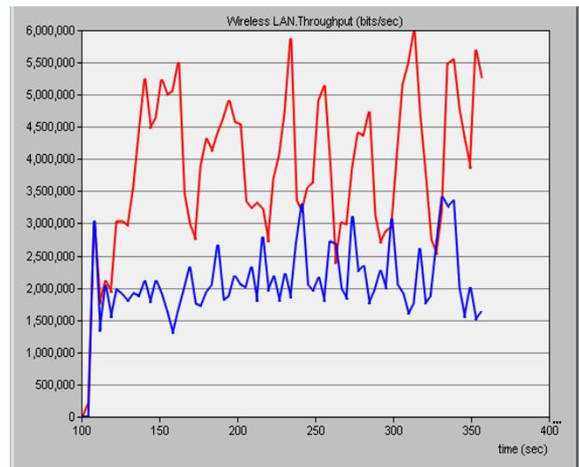
Fig. 6: The throughput of video traffic compared with AODV
