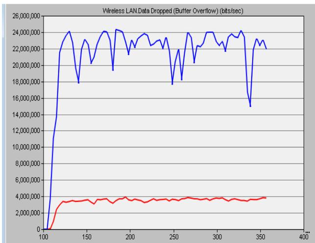
Fig. 3: Data dropped due to buffer overflow
