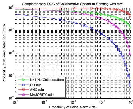
Fig. 3. Complementary ROC over Nakagami fading channel ( $N=4, \bar{\gamma}=10\text{dB}, u=5, m=1$ )
