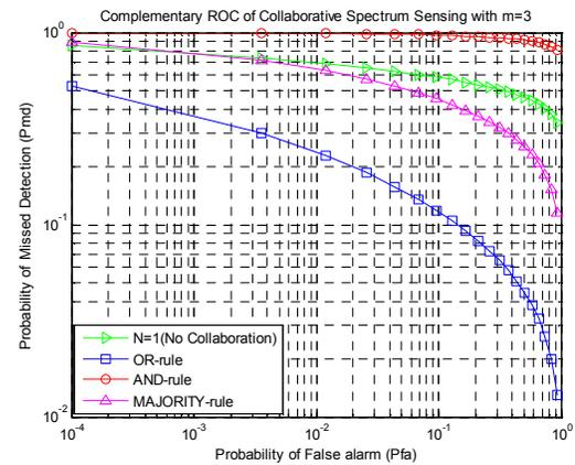
Fig. 5. Complementary ROC over Nakagami fading channel ( $N=4, \bar{\gamma}=10\text{dB}, u=5, m=3$ )
