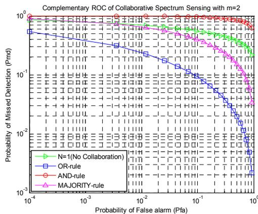
Fig.4 Complementary ROC over Nakagami fading channel ( $N=4, \bar{\gamma}=10\text{dB}, u=5, m=2$ )
