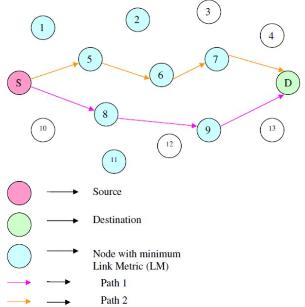
Fig. 1. Multipath Establishment using Multipath Dijkstra Algorithm
