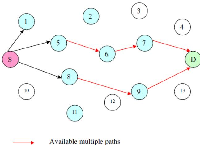
Fig. 3. Reactive Multi-path Routing
