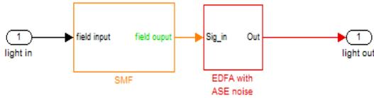
Figure 7. Single fiber transmission span
