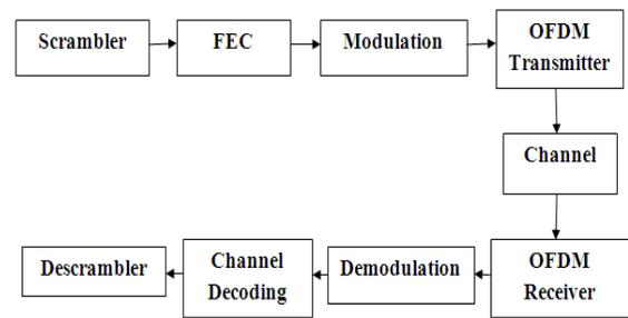
Fig. 2. Block diagram of 802.16d OFDM PHY layer
