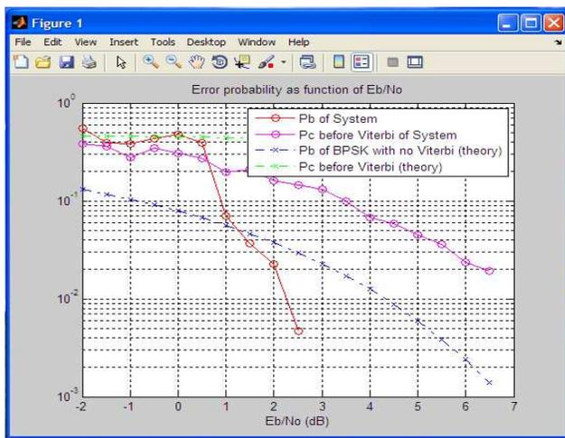
Fig. 4. Probability of Error (Bit error rate) Vs Signal to Noise ratio of BPSK
