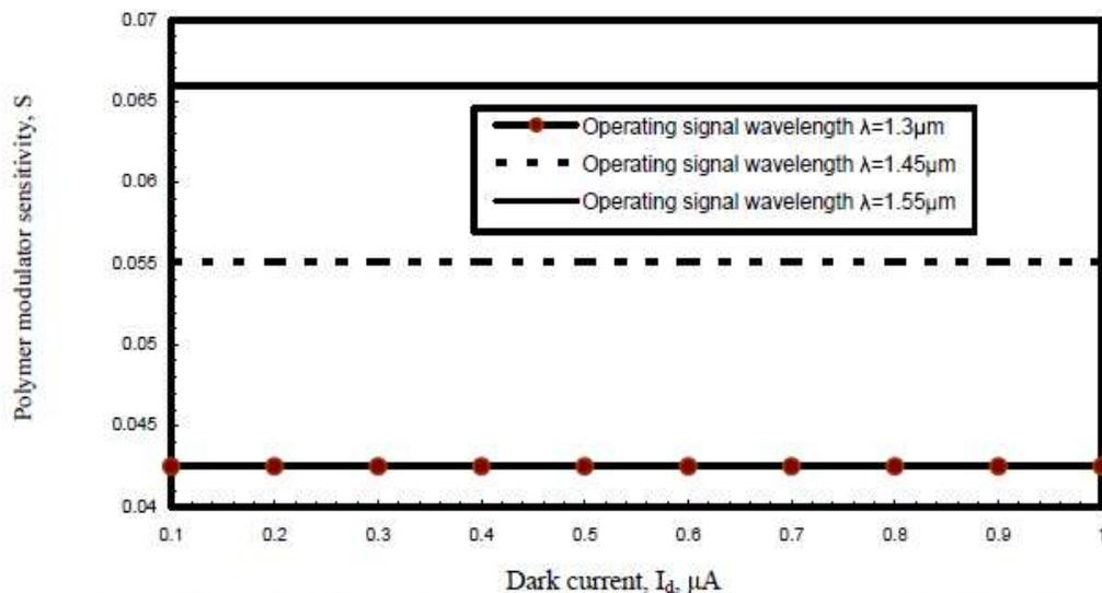
Fig. 11. Variations of polymer modulator sensitivity versus dark current at the assumed set of parameters.
