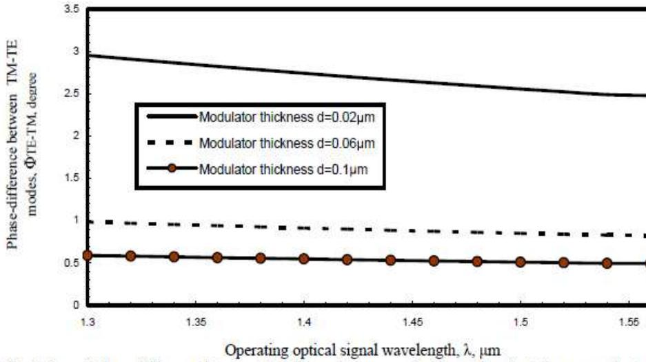
Fig. 2. Variations of phase difference between TM-TE modes versus signal wavelength at the assumed set of parameters.
