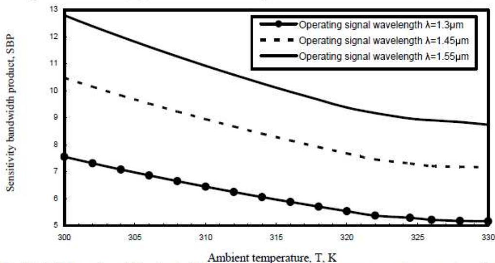
Fig. 12. Variations of sensitivity bandwidth product against ambient temperature at the assumed set of parameters.
