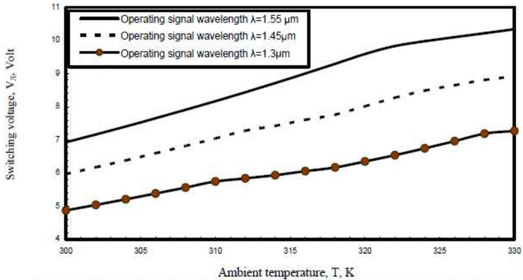
Fig. 5. Variations of switching voltage against ambient temperature at the assumed set of parameters.
