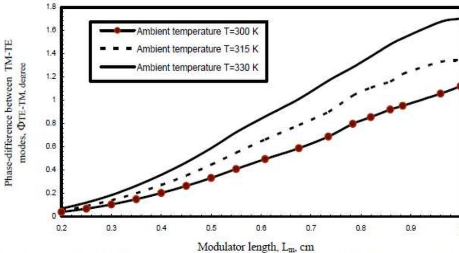
Fig. 4. Variations of phase difference between TM-TE modes against modulator length at the assumed set of parameters.
