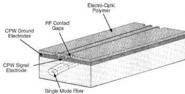
Fig. 1. High-speed traveling wave EO polymer modulator
