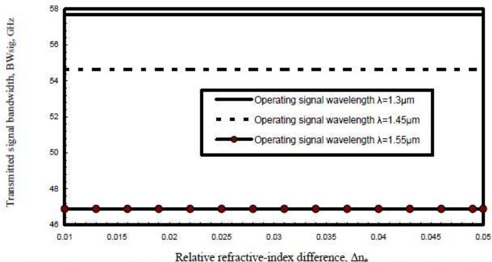
Fig. 13. Variations of signal bandwidth versus relative refractive index difference at the assumed set of parameters.
