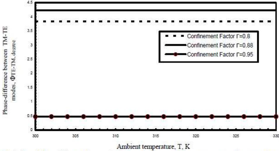
Fig. 3. Variations of phase difference between TM-TE modes versus ambient temperature at the assumed set of parameters.
