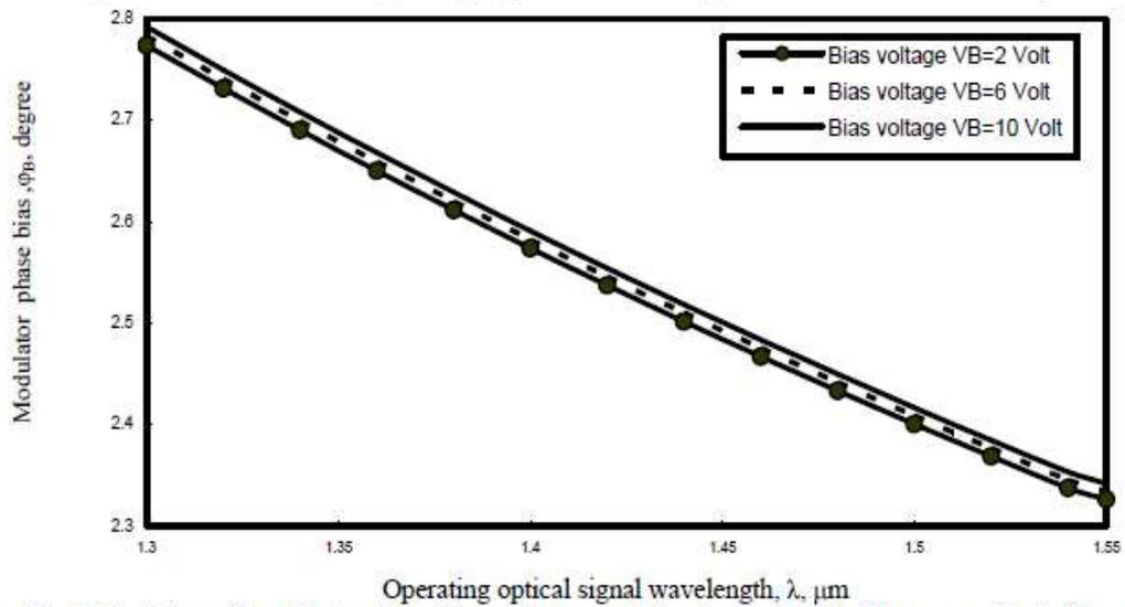
Fig. 6. Variations of modulator phase bias against optical signal wavelength at the assumed set of parameters.
