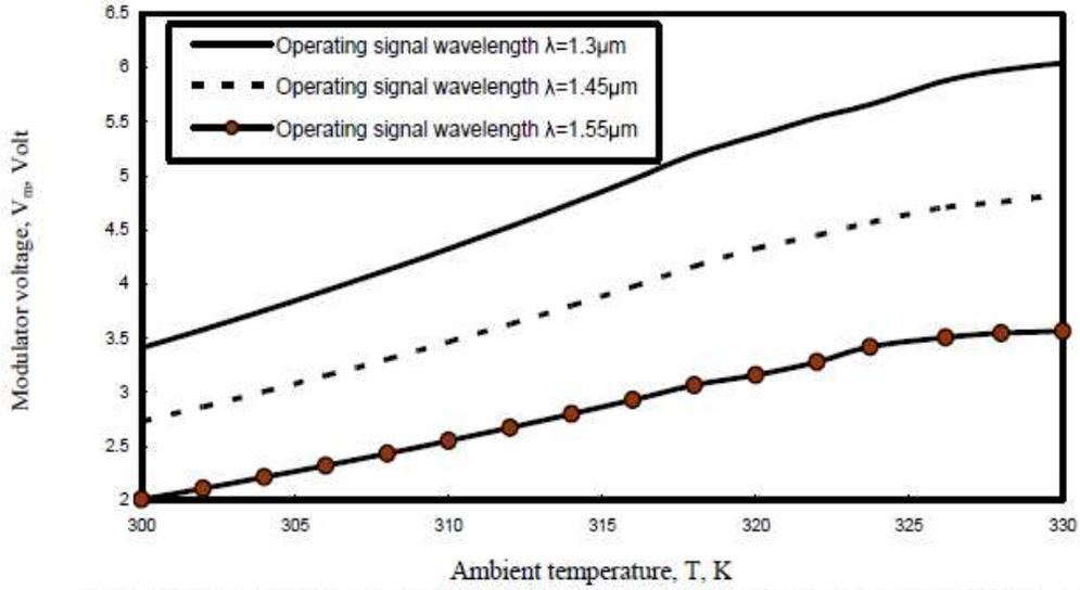
Fig. 8. Variations of modulator voltage against ambient temperature at the assumed set of parameters.
