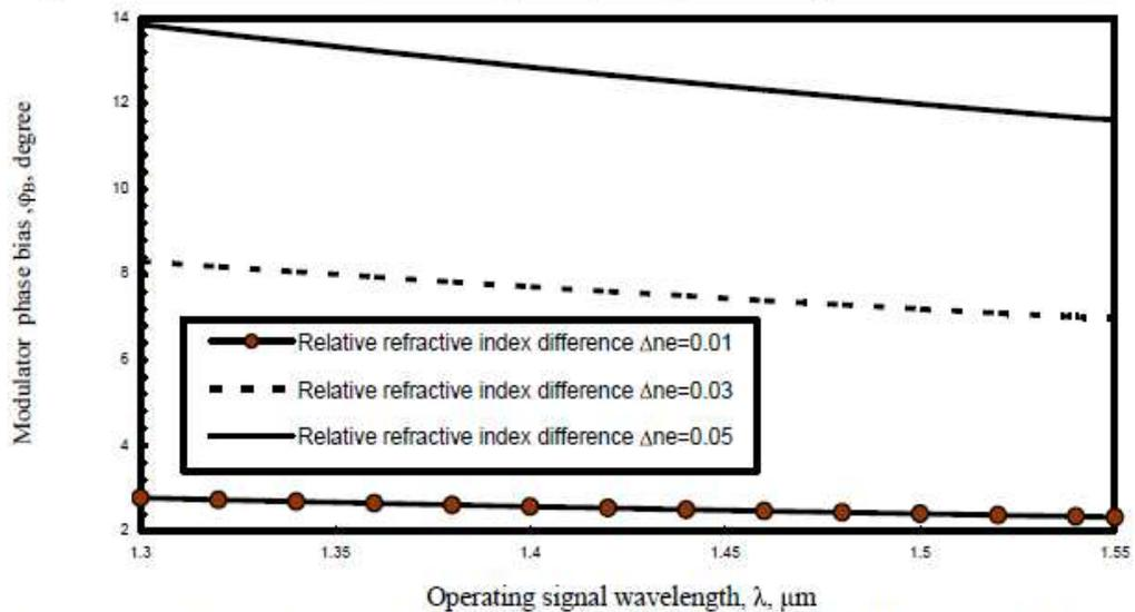
Fig. 7. Variations of modulator phase bias against optical signal wavelength at the assumed set of parameters.
