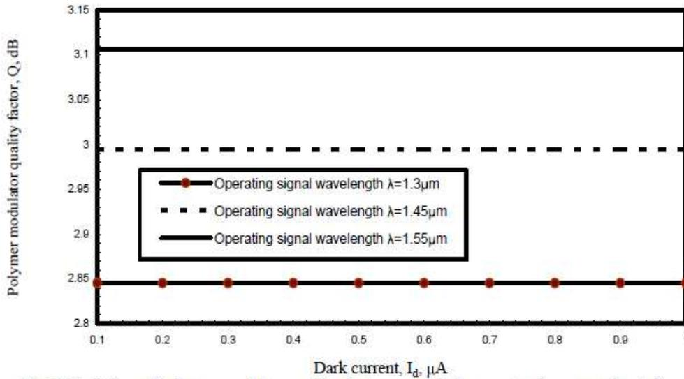
Fig. 9. Variations of polymer modulator quality factor versus dark current at the assumed set of parameters.
