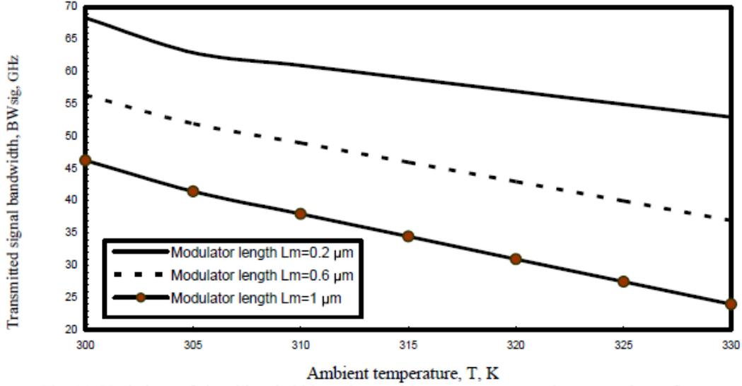
Fig. 15. Variations of signal bandwidth against ambient temperature at the assumed set of parameters.
