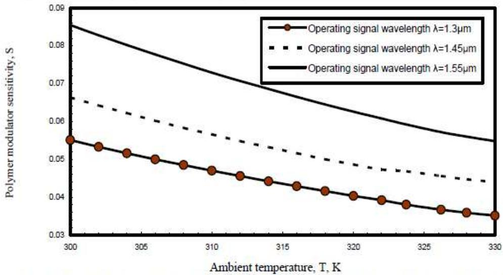
Fig. 10. Variations of polymer modulator sensitivity versus ambient temperature at the assumed set of parameters.
