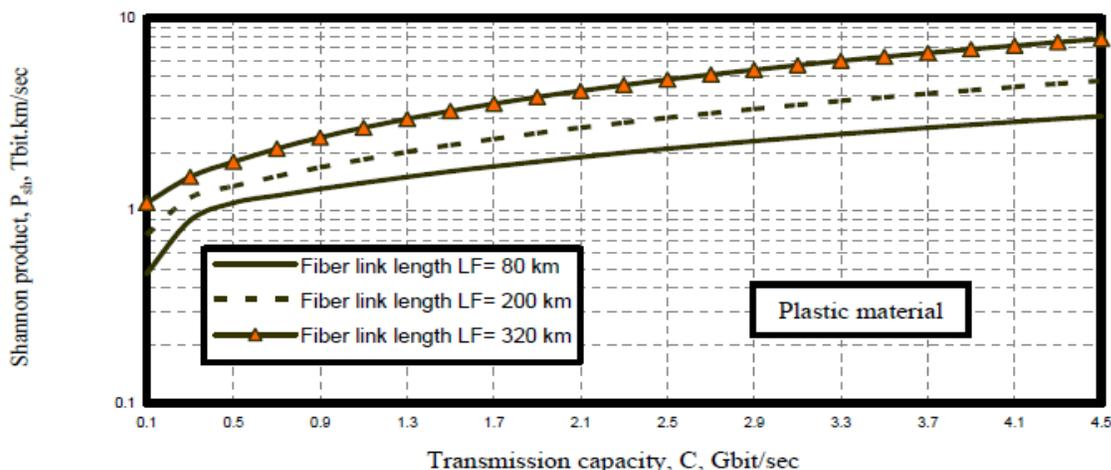
Fig. 26. Variations of Shannon product against transmission capacity at the assumed set of parameters.
