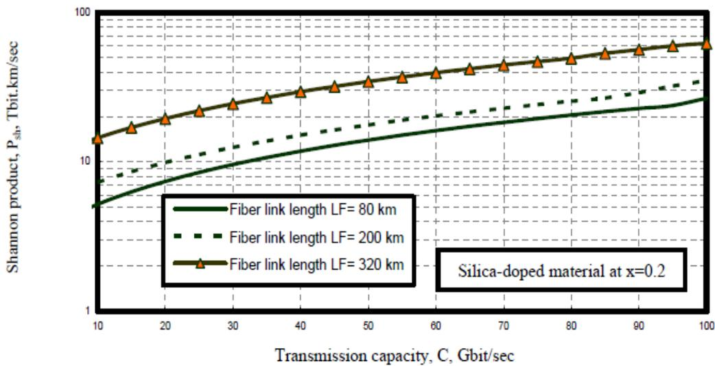
Fig. 24. Variations of Shannon product against transmission capacity at the assumed set of parameters.
