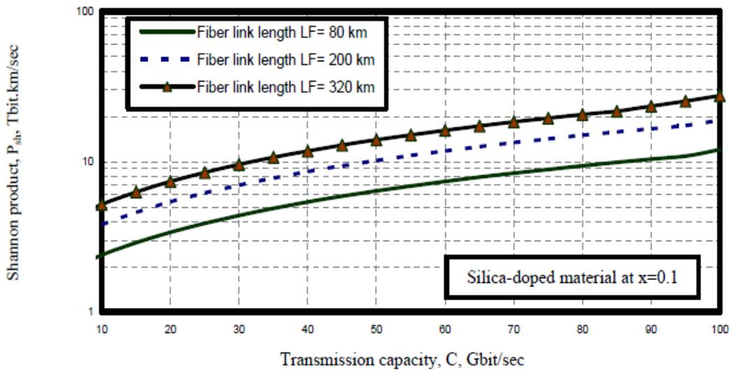
Fig. 23. Variations of Shannon product against transmission capacity at the assumed set of parameters.
