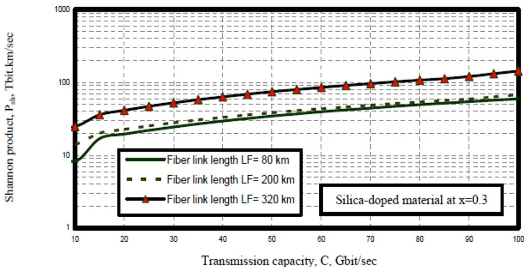
Fig. 25. Variations of Shannon product against transmission capacity at the assumed set of parameters.
